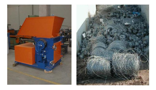
Installed to reduce wires and straps from pulp, paper, plastic and waste bales into a convenient and compact roll. The wire winder provides a solution to the problem of loose wires which can cause trip or injury hazards. The unit weighs 1380 kgs, and is simple to install. Voltage is to your requirements and an air connection of only 1.5 bar is required. The wire from up to 160 bales can be wound to a roll of 500 mm dia. by 500 mm in length. Installed power is 4 KW, absorbed power 2.5 KW.
